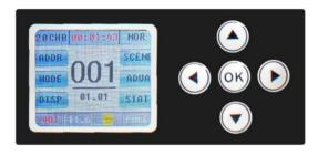
The schematic diagram of the light board is shown in Figure 3.The left side is the TFT Displayer, and the right side is the encoder button.
