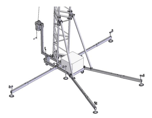
Ballast must be placed direct on the Base frame.
