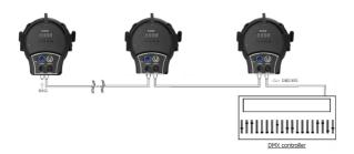
Connect the DMX-output of the first fixture in the DMX-chain with the DMX-input of the next fixture. Always connect one output with the input of the next fixture until all fixtures are connected. Up to 32 fixtures can be connected.
