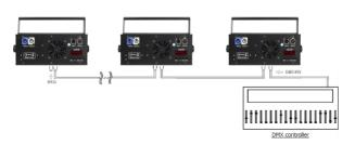
Connect the DMX-output of the first fixture in the DMX-chain with the DMX-input of the next fixture. Always connect one output with the input of the next fixture until all fixtures are connected. Up to 32 fixtures can be connected.
